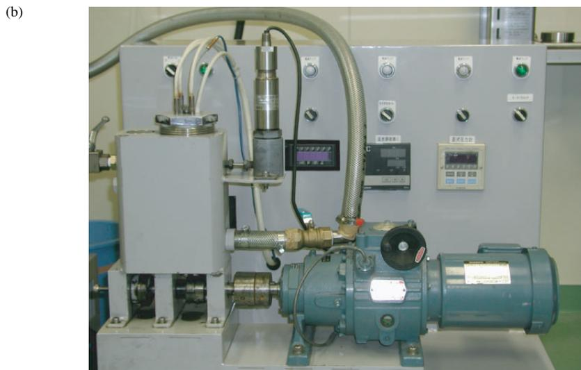
**Figure 1** Schematic diagram (a) and photograph (b) of the special hydrostatic pressure (HP) apparatus. The apparatus was used to apply arbitrary HP to cells. The Petri dishes (35 × 10 mm) were placed in a deformable Teflon pouch. Water is used as the pressure medium and pressure is transmitted to the cells through the packed Teflon pouch. The culture medium is in a gas-free environment. The temperature is maintained at 37°C by using a thermostat placed in the pressure vessel
