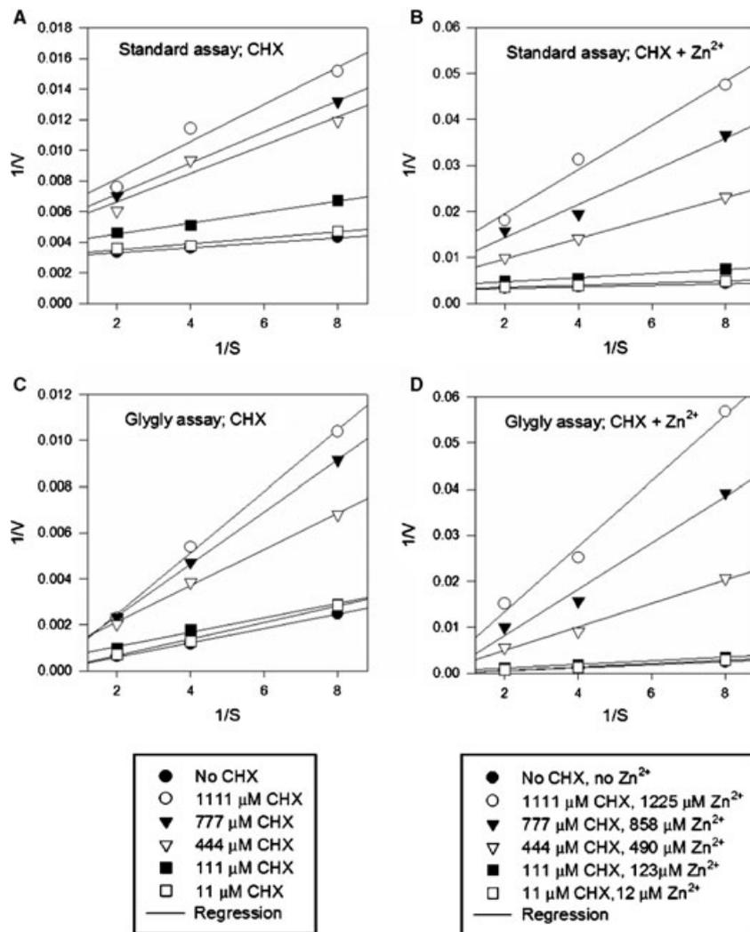
Fig. 2. Lineweaver-Burk plots of inhibition of RgpB by chlorhexidine in the presence or absence of Zn(II). The substrate was BApNA, and substrate concentrations were 0.125, 0.250, and 0.500 mM. Assay conditions and concentrations of chlorhexidine (CHX) and Zn(II) were as indicated. Lines associated with each set of points represent linear regression analysis of the respective data sets.
