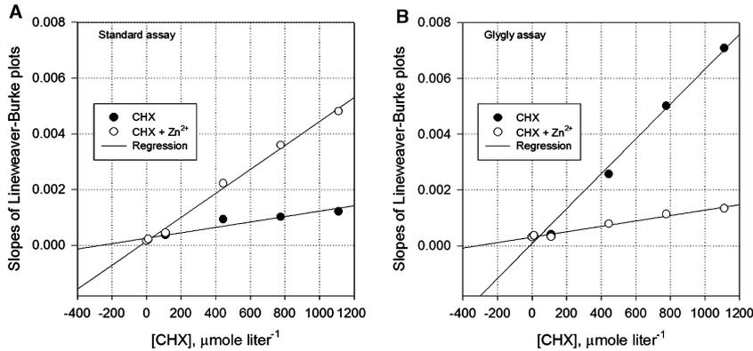
Fig. 3. Estimation of inhibition constant  $K_i$  for inhibition of RgpB by chlorhexidine (CHX), with or without Zn(II). Assay conditions were as indicated. Lines associated with each set of points represent linear regression analysis of the respective data sets.  $K_i$ 's were estimated as the negative abscissa intercepts of the regression lines.
