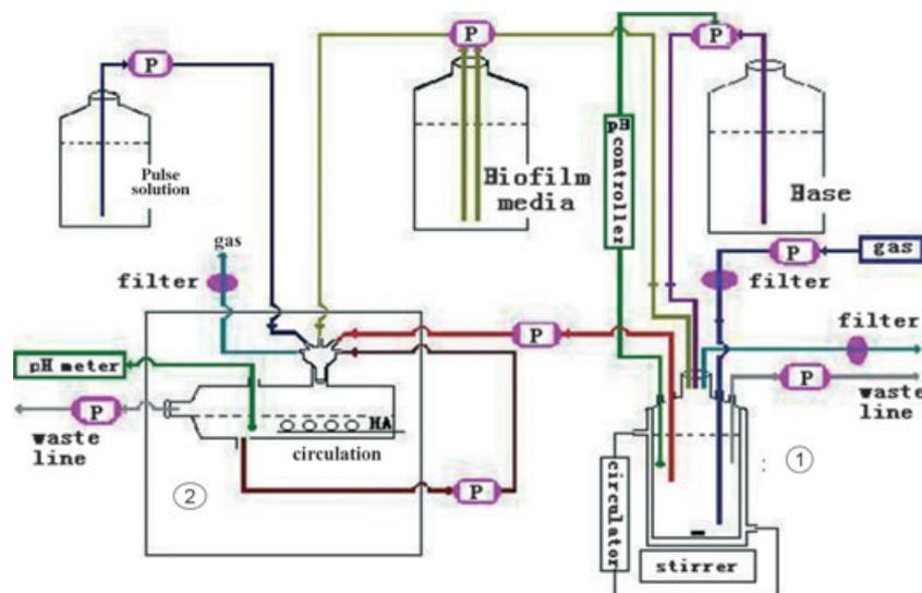
Fig. 1. Schematic diagram of the experiment biofilm system: 1, fermenter vessel; 2, flow cell.
