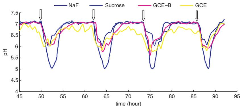
Fig. 2. The pH response in the flow cell against the pulsing. NaF = 228 p.p.m. fluoride as NaF + 25 mM sucrose; GCE = 4 mg/ml *Galla Chinensis* extract + 25 mM sucrose; GCE-B = 4 mg/ml *Galla Chinensis* extract-B + 25 mM sucrose; Sucrose = 25 mM sucrose. Arrows indicate one pulse to the flow cell.
