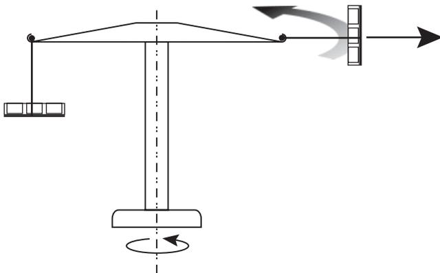
Fig. 1. Schematic drawing of the experimental setup for hypergravity simulation through centrifugation. Side view of a centrifuge. Left, the buckets in resting position. During centrifugation (right) the buckets swing out because of centrifugal force (thick arrows).
