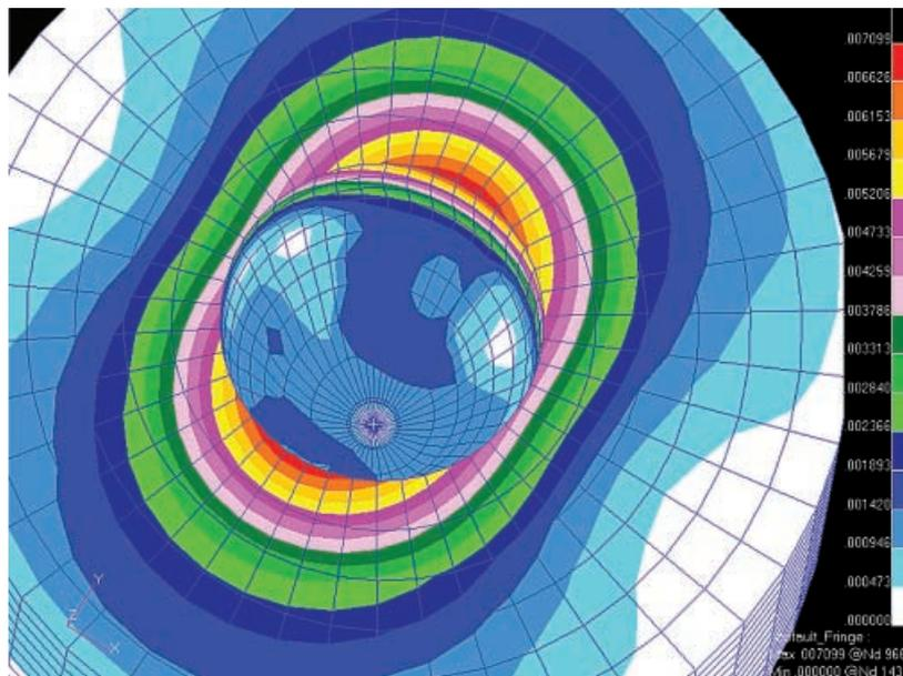
Fig. 8. Mechanical stress at root apex from intrusion – apical view.
