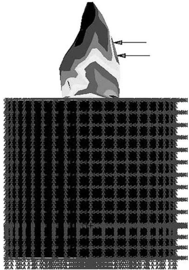
Fig. 2. Model of incisor in alveolar bone – external view. Arrows point to application of simulated orthodontic force.
