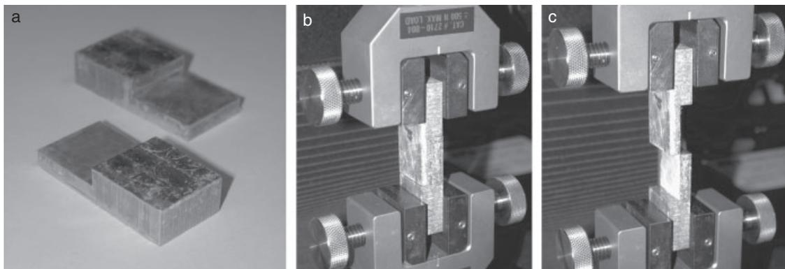
Fig. 1. Bioadhesion determination by Instron machine using fixtures: (a) Fixtures; (b) loaded fixtures before test; (c) after test.
