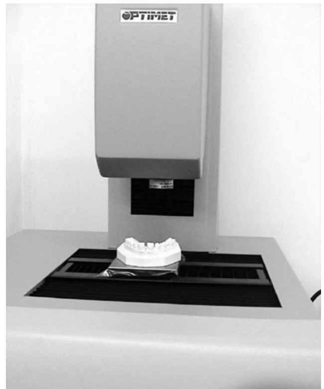
Fig. 1. Optimet 3D scanner with the 'ConoProbe' Holographic sensor.
