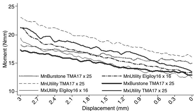
Fig. 3. Graph depicting the variation of posterior moments in the sagittal plane ( $M_y$ ) with vertical displacement from 0.0–3.0 mm (0.5 mm increments) for the biomechanical systems included in the study.
