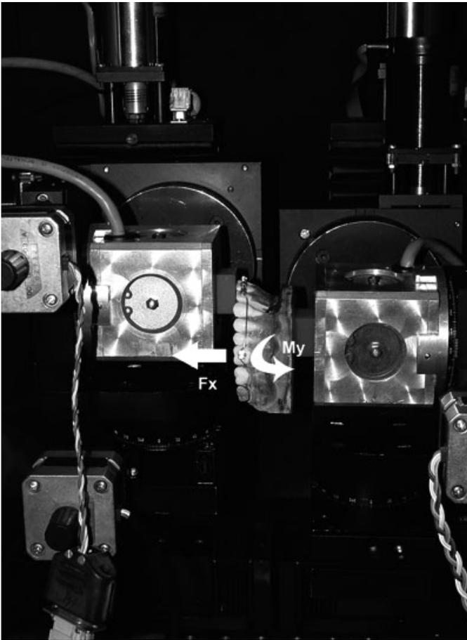
Fig. 1. The acrylic Frasaco model mounted to the positioning tables of the OMSS.
