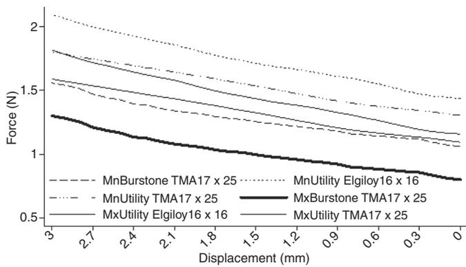
Fig. 2. Graph depicting the variation of extrusion forces ( $F_x$ ) with vertical displacement from 0.0–3.0 mm for the biomechanical systems included in the study.
