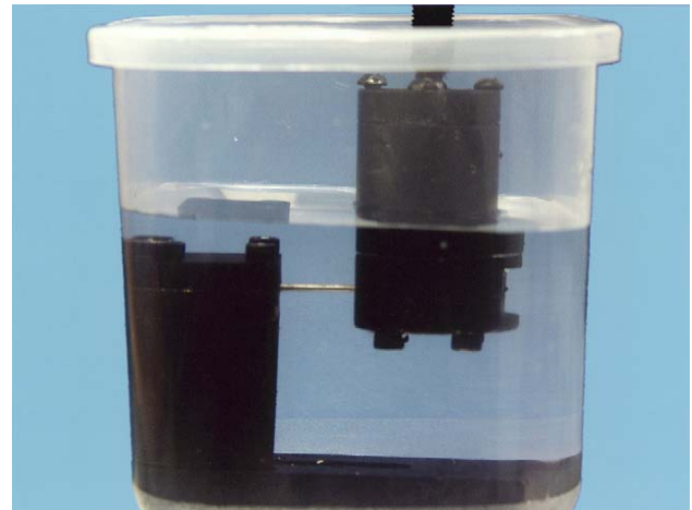
Fig. 2. Plastic apparatus with fluoridated saliva for corrosion-fatigue test.
