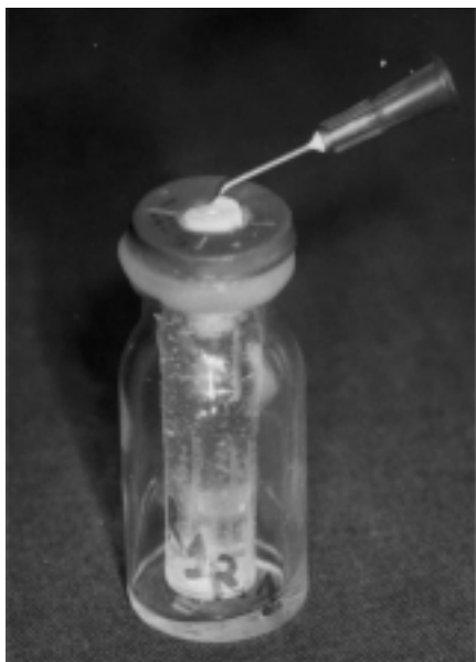
Fig. 1 System using a mounted tooth in a flask. A vial containing distilled water was placed in the glass flask and then the cap of the flask with a root inside its perforated area was placed in this system so that the apex was inside the water and the cap was sealed with glue.
