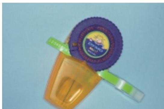
Fig. 2 A manual label marker (Dymo Mini) used for preparation of the plastic pattern.
