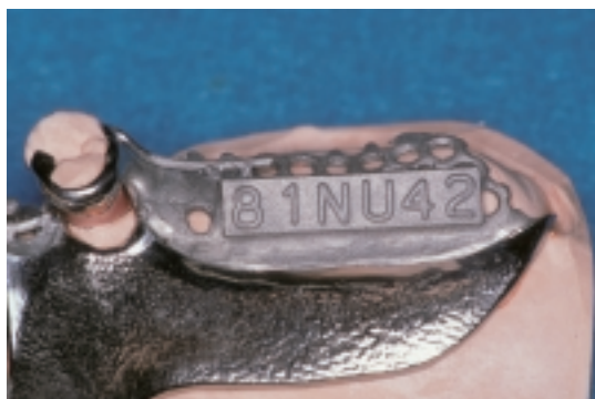
Fig. 4 The cast framework of the partial denture made from Ti-6Al-7Nb alloy. The embossed letters were clearly reproduced.
