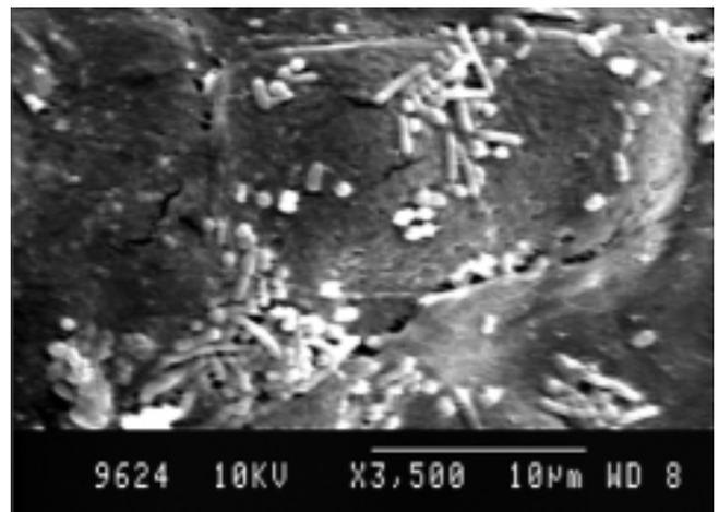
Fig. 11 SEM of bacteria adhering to CS after 14 days.
