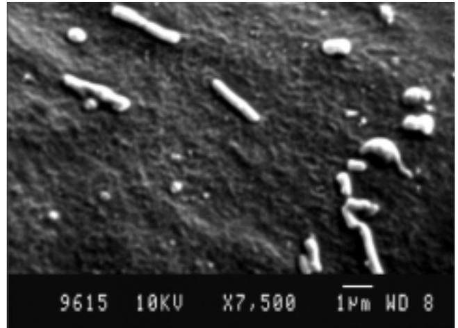
Fig. 10 SEM of bacteria adhering to SL after 14 days.
