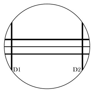
Fig. 1 Schematic illustration of the stainless steel test die showing the distance between the inner profile of Line d1 and the inner profile of Line d2 (d1-d2 distance). The width of vertical lines (d1 and d2) is 0.075 ± 0.008 mm, whereas the distance between the lines d1-d2 is 25 mm.
