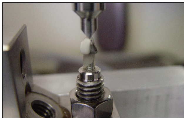
Figure 2. Instron custom holder and application of force to veneers of veneered stainless steel crowns.
