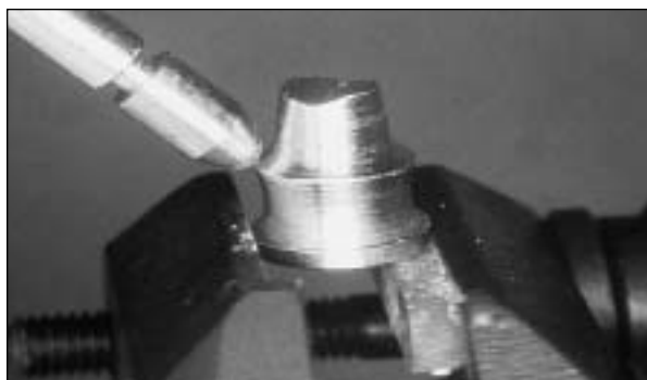
Fig 1 Sapphire probe stylus with the brass die in situ (chamfer preparation).
