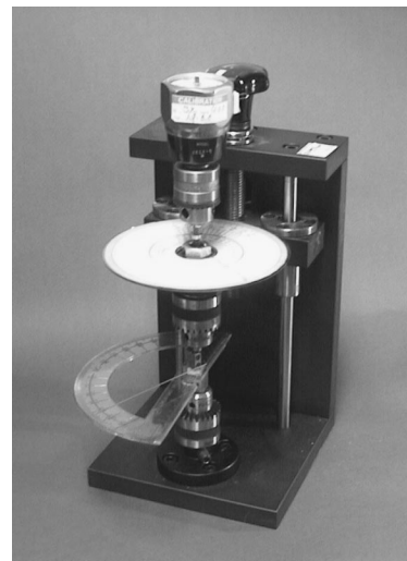
FIGURE 2. The torque gauge measurement system used in the study.
