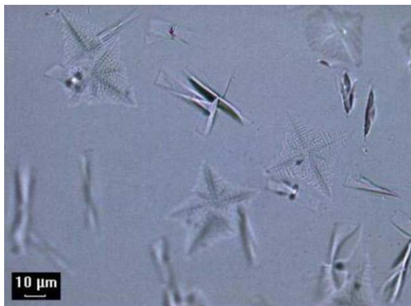
Figure 2 Light microscope image of the 950 °C specimen displaying the morphology of leucite and sanidine crystals ( \times 50 ).
