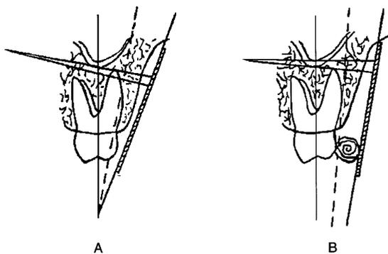
Fig. 4 When exposing films of maxillary molars, the standard bisecting angle technique (A) often produces superimposition of the zygomatic process over root apices. Placing a cotton wool roll on the inferior border of the film produces a more parallel relationship between teeth and film, allowing a reduction in the vertical angulation (B), so decreasing the incidence of superimposition (Rosa & Tavares 1988). Alternatively, a film holder and beam aiming device can be used.
