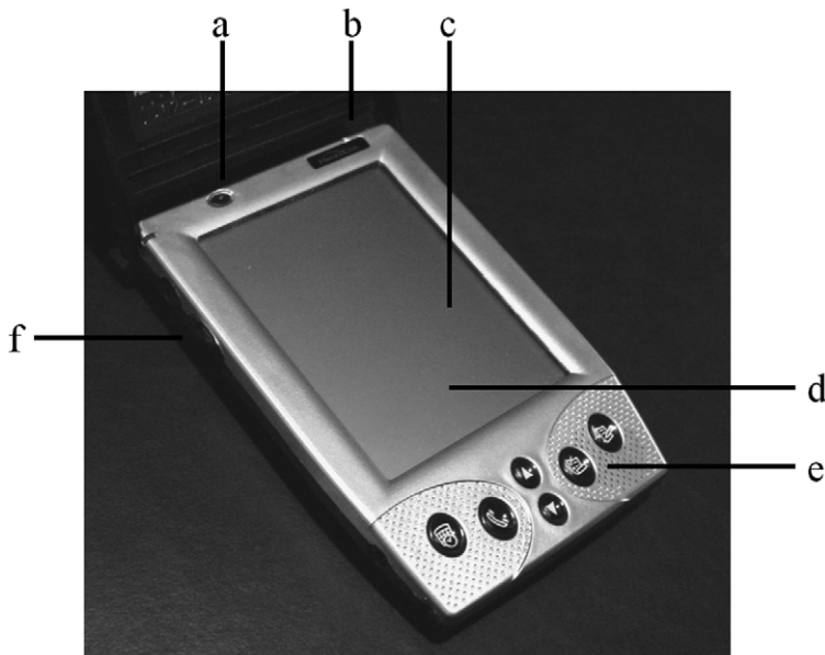
Fig. 1. Front view of a PDA. Features include (a) the power button, (b) microphone, (c) screen, (d) writing area, (e) quick access buttons, and (f) jog wheel.
