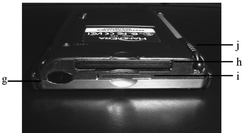
Fig. 3. Top view of a PDA. Features include (g) the infrared port, (h) compact flash expansion slot, (i) secure digital expansion slot, and (j) stylus.
