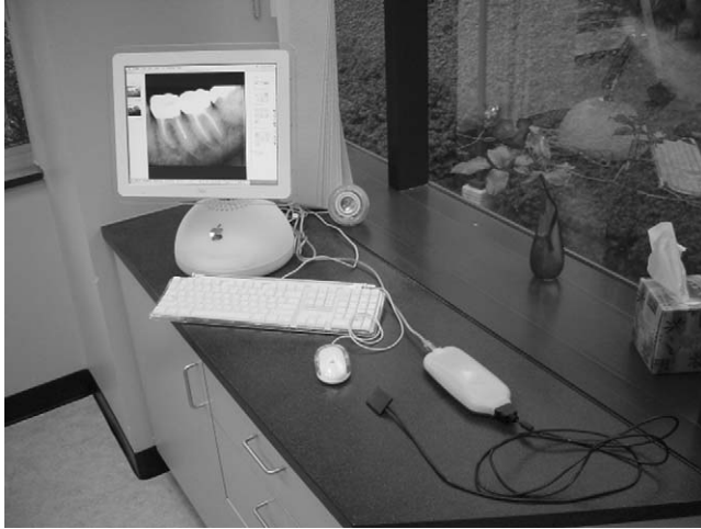
Fig. 5. Digital xray system: wired sensor connected to a USB interface with the computer. The exposed sensor produces an image on the computer display for viewing and manipulation.
