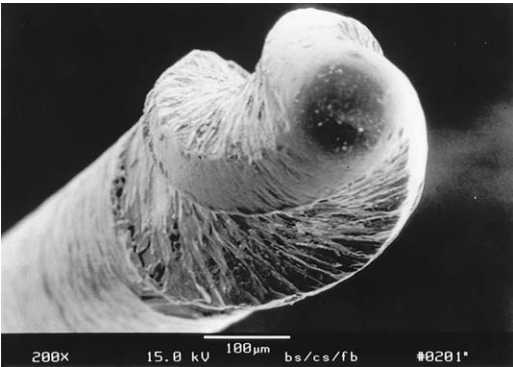
Fig. 3. SEM photomicrograph of a LightSpeed cutting head showing the noncutting pilot tip, radial lands, spiral grooves, and part of the taperless shaft in an unusual perspective (original magnification ×200).
