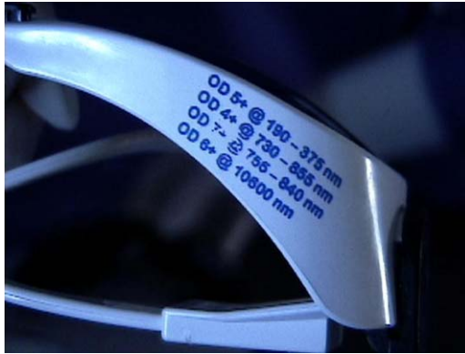
Fig. 2. Information about eye protection printed on the safety glasses must include the optical density and protected wavelengths, as shown.
