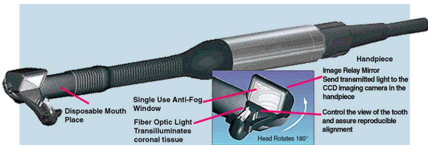
Fig. 3. The proximal or occlusal mouthpiece is placed over the tooth in question, allowing light to be shined from one surface, through the tooth, and captured on the opposite side using a CCD camera in the DIFOTI handpiece. (Courtesy of Electro-Optical Sciences, Irvington, New York; with permission.)
