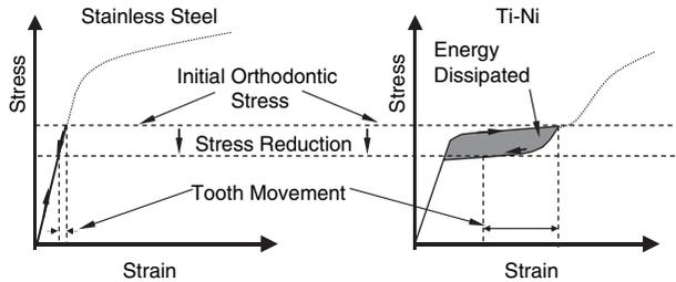
Fig. 7. Comparison of stress strain curves for stainless steel and a superelastic Ti-Ni alloy that exhibits a plateau resulting from stress-induced phase transformation. After an applied orthodontic stress, more tooth movement can be accommodated by a Ti-Ni wire compared with a stainless steel wire for a given decrease in applied stress. This schematic also illustrates the energy dissipation that is achieved by the Ti-Ni alloy when deforming in the superelastic plateau region.
