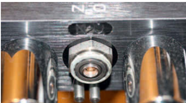
Figure 14-11 Pins, which are located on yoke of inhalation sedation unit, are aligned to permit attachment of only one compressed gas.
