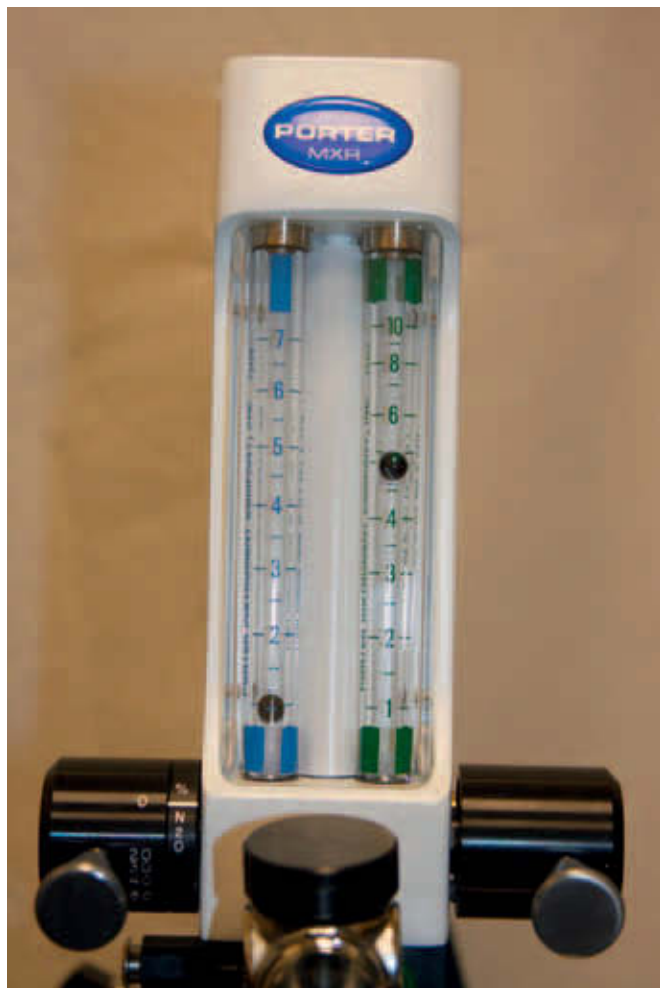
Figure 15-8 Constant liter flow technique: O 2 flow decreases 1 L/min to 5 L/min, N 2 O flow increases 1 L/min to 1 L/min, and N 2 O percentage equals 16.6%.
