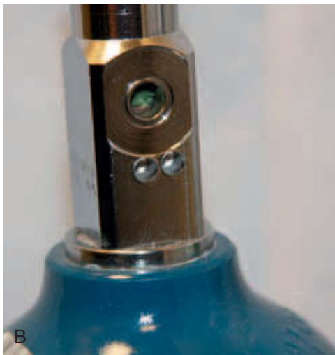
Figure 14-10 Pin index safety system for O 2 (A) and N 2 O (B). Large orifice on top of cylinder permits gas to exit cylinder. Smaller holes below are pin indexed for specific compressed gas.
