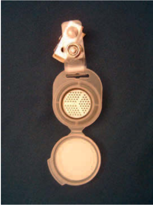
Figure 17-3 N 2 O monitoring device is worn by nitrous oxide oxygen sedation providers to evaluate occupational exposure.
