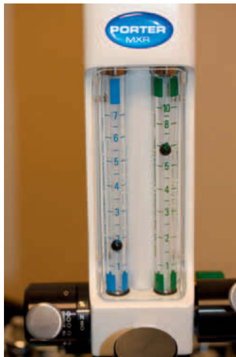
Figure 15-9 Constant O 2 flow technique: O 2 flow remains constant at 6 L/min, N 2 O flow is raised 1 L/min, and N 2 O percentage equals 14.3%.
