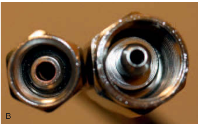
Figure 14-34 A , Back of inhalation sedation unit. Note different diameters of N 2 O (right) and O 2 (left) connectors. B , Diameter index safety system. Diameter and threading of N 2 O coupling (right) differ from those of O 2 coupling (left), thus preventing accidental attachments to wrong side of inhalation sedation unit.
