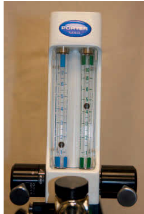
Figure 15-10 Constant liter flow technique; subsequent changes in gas flow every 60 to 90 seconds are an 0.5-L/min O_2 decrease and 0.5-L/min N_2O increase.
