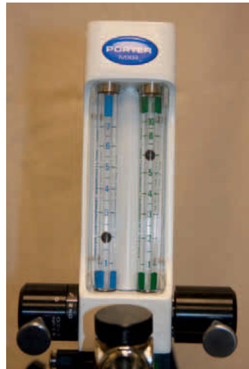
Figure 15-11 In constant O_2 flow technique, subsequent changes in gas flow are a 1-L/min increase in N_2O every 60 to 90 seconds.
