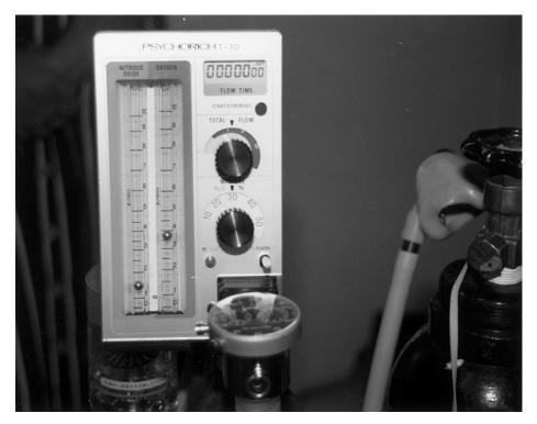
Figure 7-2  $N_20/0_2$  machine capable of calculating patient charges according to the amount of gas used. (Courtesy of Dr. Yuzuru Kaneko, Dept. of Dental Anesthesiology, Tokyo Dental College, Tokyo, Japan.)
