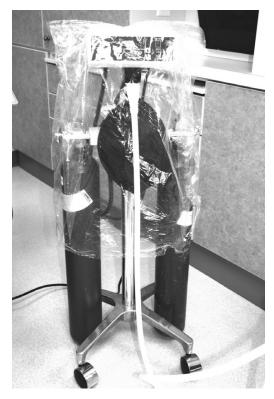
Figure 13-5 Bag barrier for disinfection.
