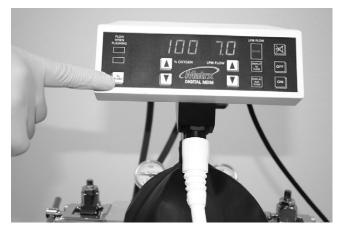
Figure 13-9 Begin the flow of oxygen at an average rate per minute and fill the reservoir bag two-thirds full by use of the  $0_2$  flush button.
