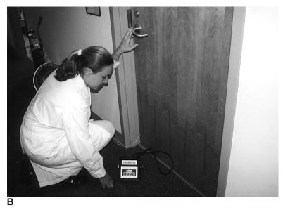
Figure 17-9 A and B, Monitoring airflow with an electronic micromanometer.
