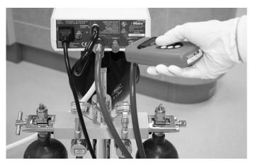
Figure 13-1 Checking connections on the flowmeter for leaks.
