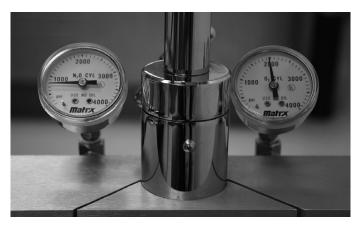
Figure 13-3  $N_2 0 \mbox{ and } 0_2$  pressure gauges indicating cylinder contents.
