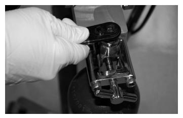
Figure 13-2 Open the  ${\rm O}_2$  tank by turning the value on top of the cylinder.
