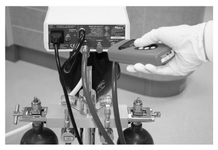
Figure 17-8 Checking connections on the flowmeter for leaks.
