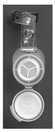
Figure 17-3 Time-weighted average dosimetry badge. (Courtesy of Assay Technology, Pleasanton, California.)
