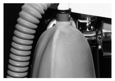
Figure 17-6 N<sub>2</sub>O leak potential resulting from the breakdown of certain materials.
