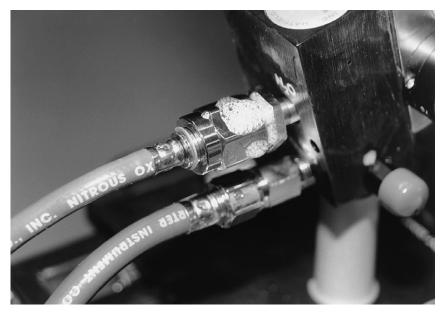
Figure 17-7 Soap and water solution used to test for  $N_2O$  leaks.
