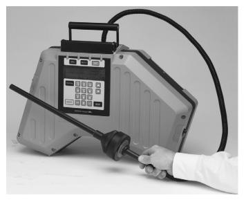
Figure 17-2 Infrared spectrophotometer. (Courtesy of Thermo Environmental Instruments, Inc., Franklin, Massachusetts.)
